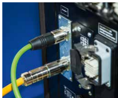
Servo cables: Motor- and encoder cables connected to the hotrunner controller
